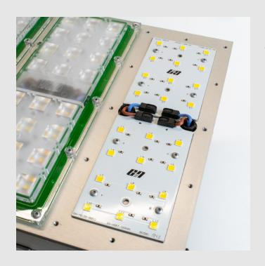
IMPORTANT NOTE: Make sure the brown and blue cables are inserted into the exact connector they were removed from.
