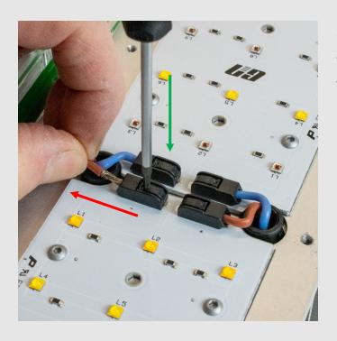
Caution: Use only the required force when depressing the electrical connector – too much force can damage the part.
